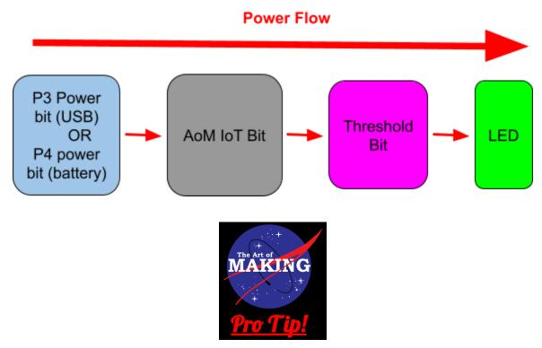
Dust your Littlebits connections with a microfiber cloth to ensure a sound electrical connection and use LittleBits magnetic <u>shoes</u> to keep the circuit from breaking connection and resetting.
