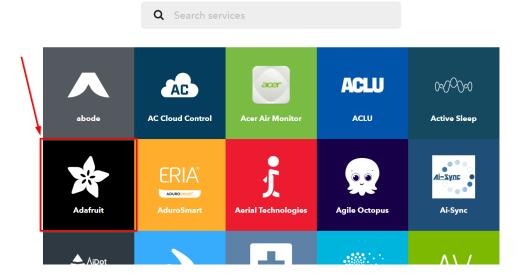
Authorize the sign-in prompt on IFTTT and select "Monitor a feed on Adafruit IO" as your trigger. Add the AoM Cloud's Adafruit IO account name (**AoM IoT Bit**,) AoM Cloud's feed name (**cloud - Feed {X}**), set the relationship as "**equal to**," and select "**HIGH**" as the value. This will trigger the "If this" portion of the widget any time the IoT bit uploads a HIGH value to Adafruit IO.
