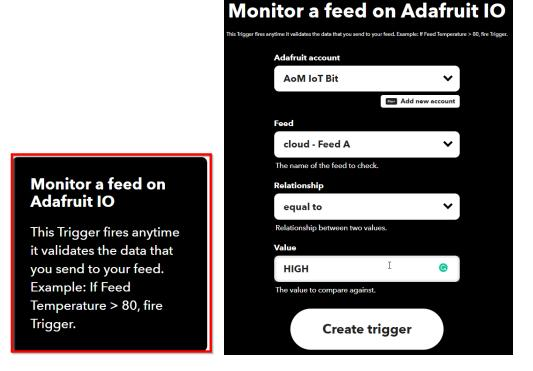
In the "Then That" field of the widget, select any web service that you want to interface to - it's up to you! A simple "Hello World" test is the Google Tasks service, which allows you to create a task every time the Adafruit IO cloud receives a high value (i.e. *IF* Adafruit IO gets a high value, *THEN* create a Google Task.) But you're only limited by your imagination - and the limits of the free IFTTT account, of course.
