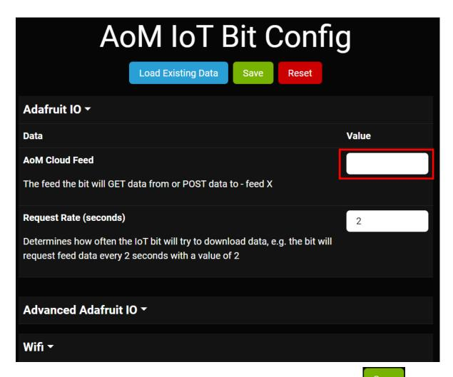
Enter in the feed that you'd like to connect your IoT Bit to (A-F), hit the button, and load the SD card back into the IoT Bit.
