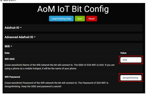
Enter in your WiFi credentials, hit the button, and load the SD card back into the IoT Bit. When you boot it back up, the IoT bit will indicate a successful WiFi connection with a green illuminated LED.
